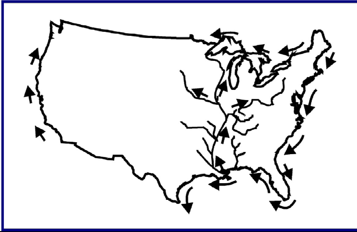
Figure 2 – CDB - Conventional Direction of Buoyage Graphic
