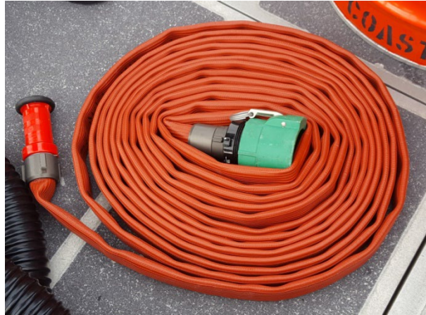
Figure 5-15 Fire Fighting Hose
