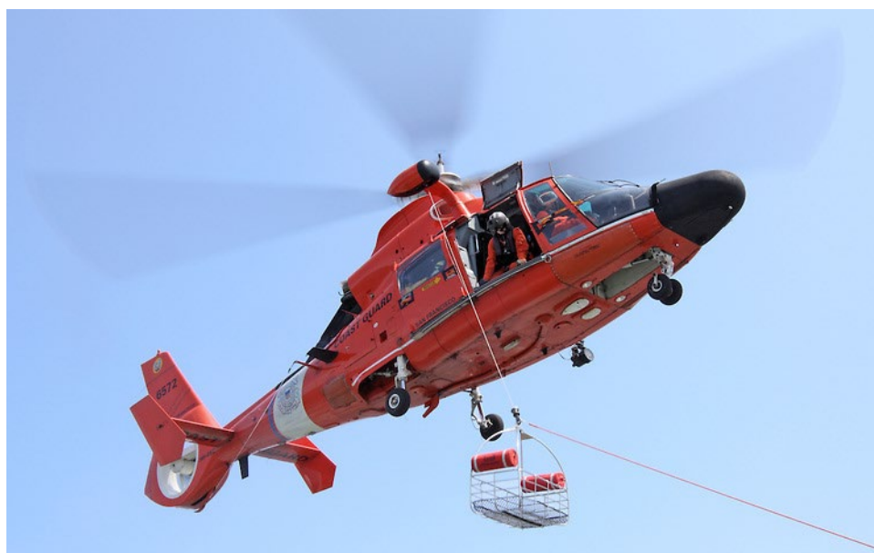
Figure 6-12 M/J Rescue Basket Going Down
