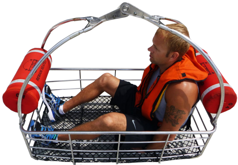
Figure 6-15 M/J Rescue Basket with Person Properly Positioned and Ready for Hoist
