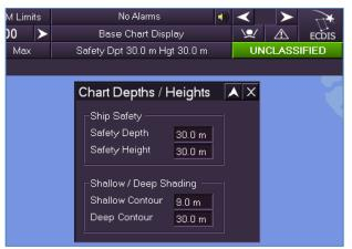
Figure 2-2: Safety Depth display
