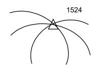
Electronic fix using radar ranges
