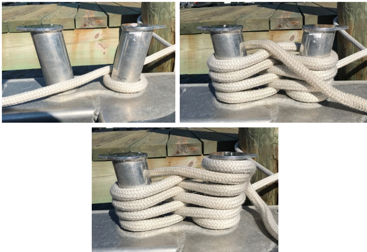
Figure 2-34 Securing a Line to Paired Bitt
