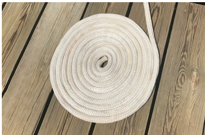
Figure 2-7 Flemishing a Line
