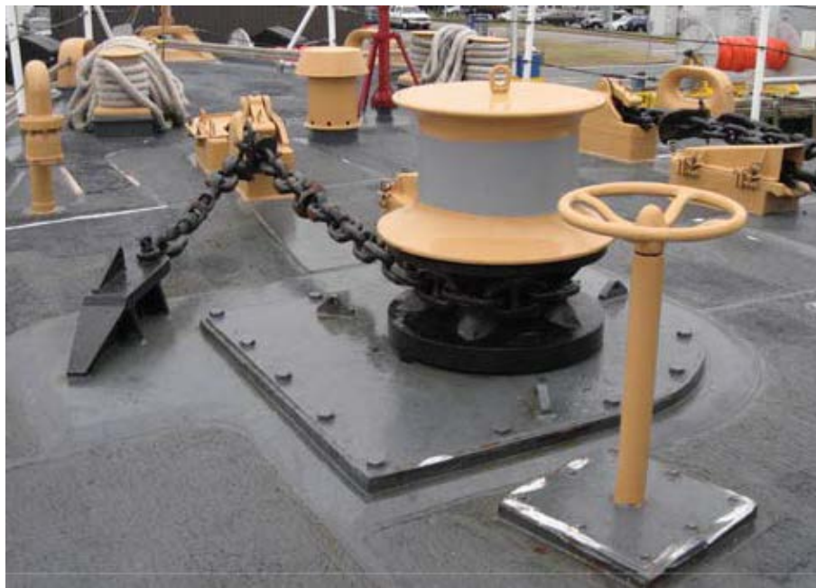
Figure 3-10 Vertical shaft windlass
