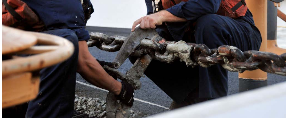
Figure 3-20 Passing the stopper
