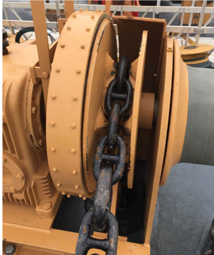
Figure 3-7 Wildcat, with brake, and stud-link chain in whelps
